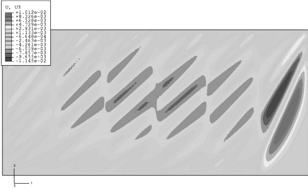
b) Excessive shear buckling at the end of the analysis, after 102 load increments
