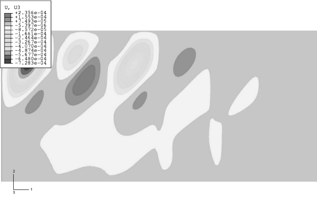
a) Onset of shear buckling, after 13 load increments
